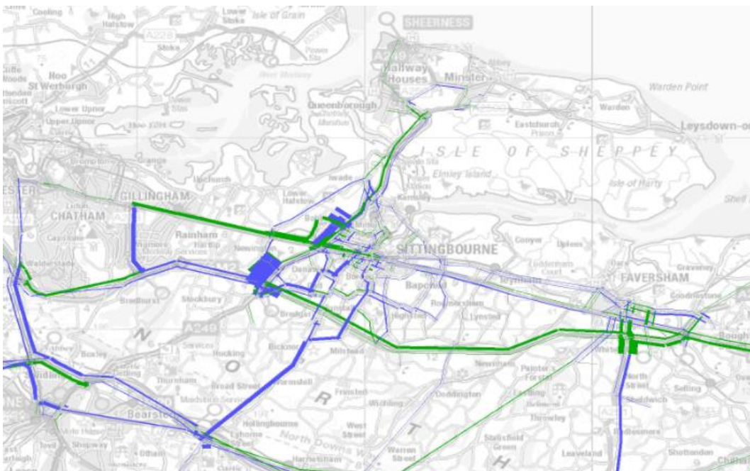
Figure 8-19 Model flow difference between 2037 Scenario 3 and Scenario 2 – Sittingbourne PM
