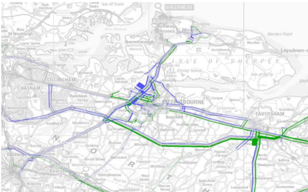
Figure 8-17 Model flow difference between 2037 Scenario 3 and Scenario 2 – Sittingbourne AM
