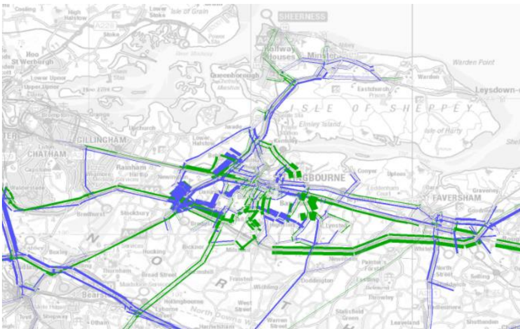
Figure 8-15 Model flow difference between 2037 Scenario 4 and Scenario 1 – Sittingbourne PM
