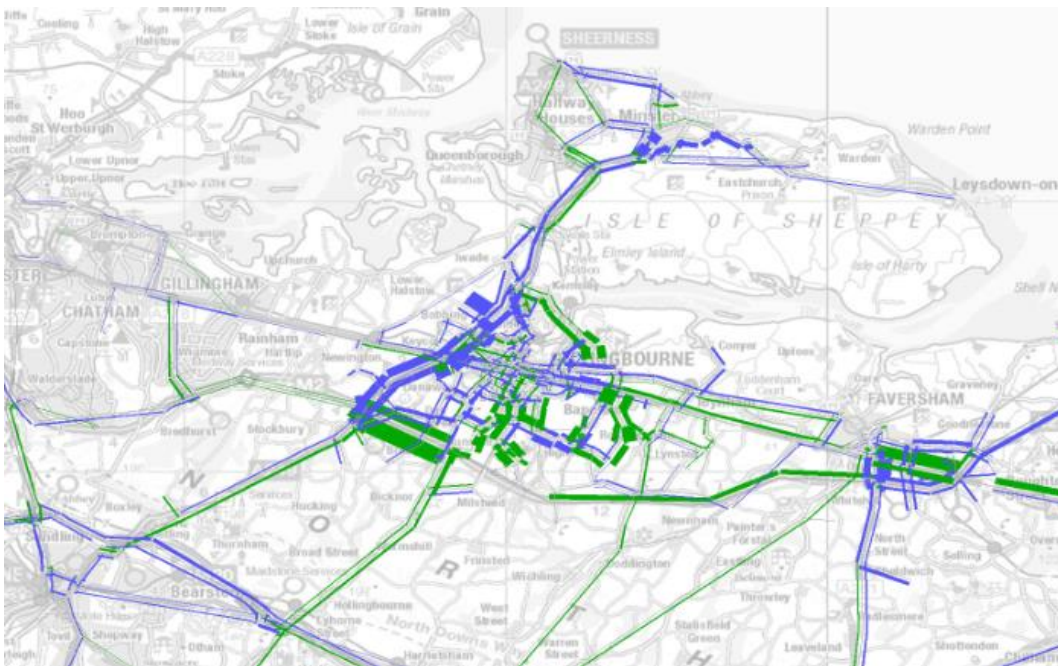
Figure 8-13 Model flow difference between 2037 Scenario 4 and Scenario 1 – Sittingbourne AM
