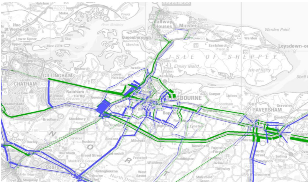
Figure 8-11 Model flow difference between 2037 Scenario 3 and Scenario 1 – Sittingbourne PM
